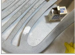
Pour baking soda over the crack until the glue is completely covered under a layer of baking soda.
