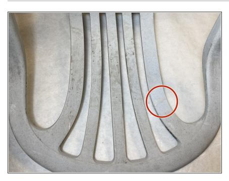
The crack has been repaired!
