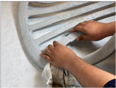
Lay the broken chair such that the crack is parallel to the floor.
