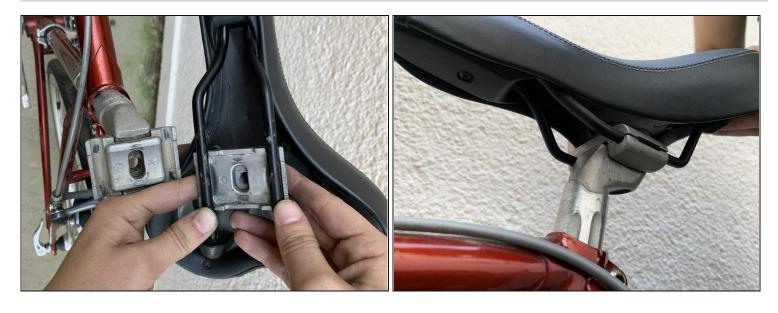
• Position the new seat's rails into the seat clamp with the clamp lying approximately flat and in the center of the rails.
