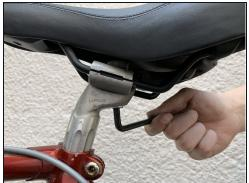
• Turn the bolt clockwise with the hex key to partially tighten the seat so it is stable enough to hold your weight.
