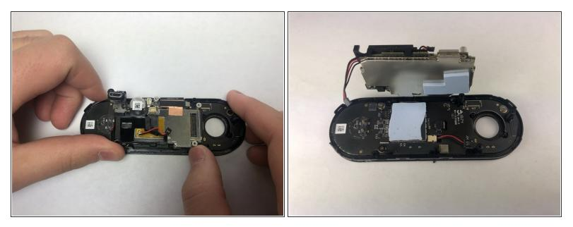
• Holding the device as shown push the circuit board away from you and up to free it from the clips.
