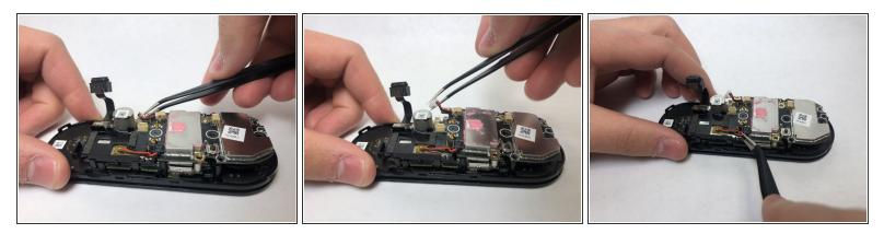
• Remove the plug connecting the camera to the device.
