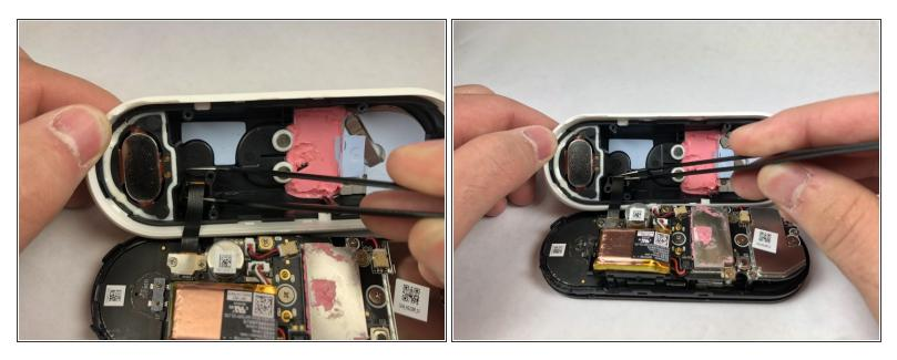
• Grip the connector with the tweezers as shown and pull it away from the casing.
