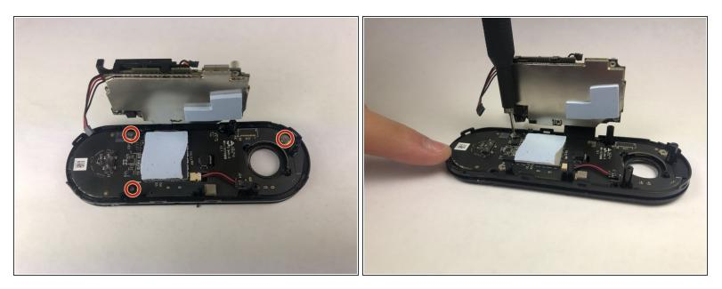
Use the Phillips #000 screwdriver to remove the three screws holding the last circuit board to the black plastic housing.
