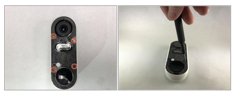
Peel back the cover stickers and use the Phillips #000 screwdriver to remove the four screws.
