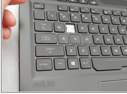
• Use the plastic opening tool to lift up on the side of the key until it pops out.
