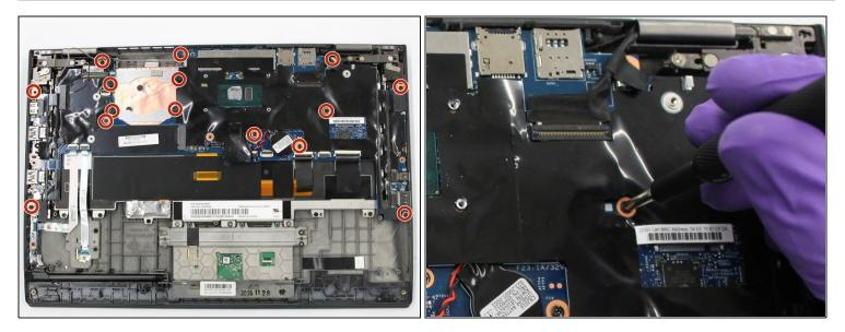
• Using the Phillips #1 screwdriver, remove sixteen 4.5mm screws.
