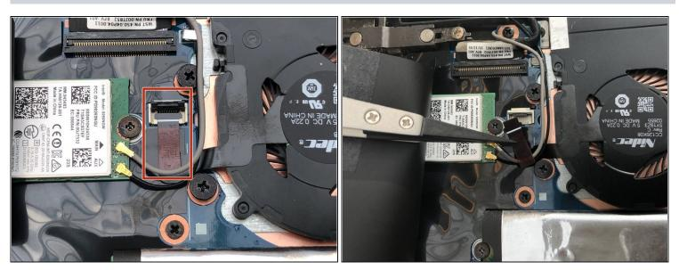
• Using tweezers, pull the plastic strip out.
