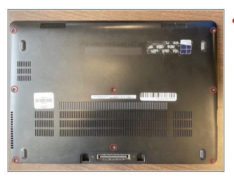
Remove the eight 4 mm screws on the back cover using a Phillips #0 screwdriver.
