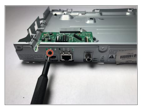
Use the Phillips #00 screwdriver to remove the 9.7mm screw holding the HDMI port in place on the outside of the case.
