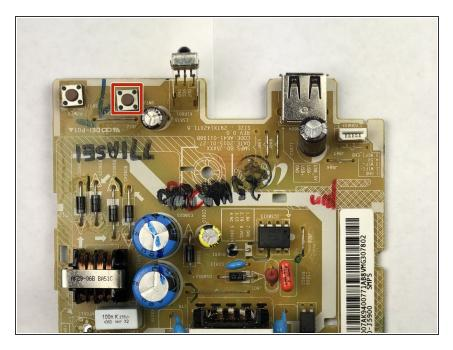
Locate the Open Button on the circuit board.
