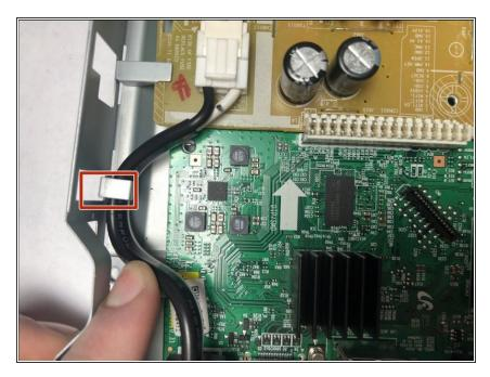
Move the power cord out from under the metal tab on the side of the case.
