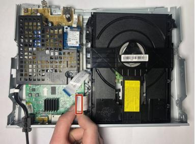
Disconnect the two ribbons that connect the disc drive to the motherboard.
