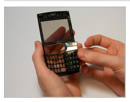
Peel back the rubber keypad from the front casing.
