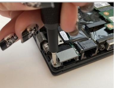
Unscrew the single, 3.0 mm screw with a Phillips #1 screwdriver bit that holds the charging port housing into place.
