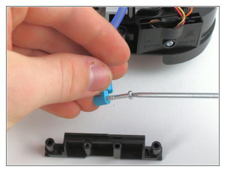
Continue unscrewing the 16 mm screw until it comes out of the nozzle.
