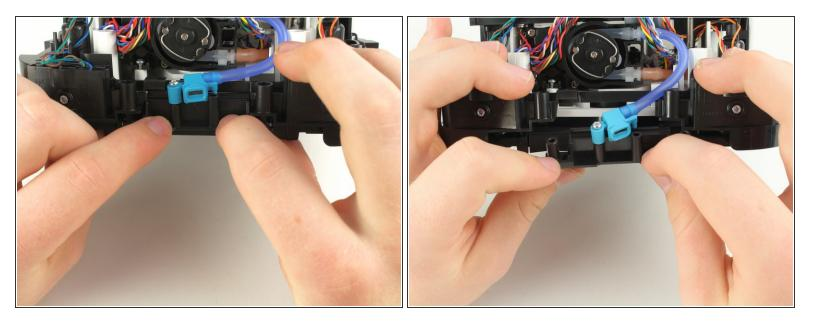
• Pull the nozzle assembly away from the body of the robot.
