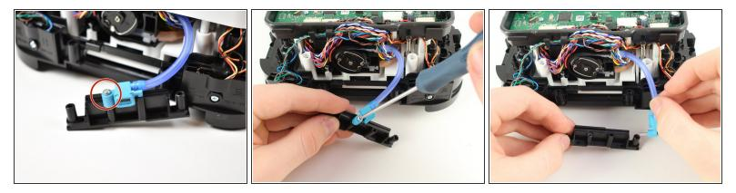
• Using a Phillips #1 screwdriver, remove the 16 mm screw that holds the nozzle in place.
