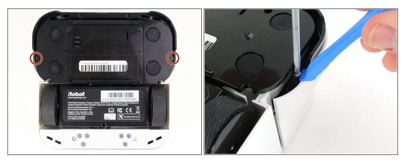
Use a Phillips #1 screwdriver and an iFixit opening tool to remove the two 15.0 mm screws on the front sides of the robot.
