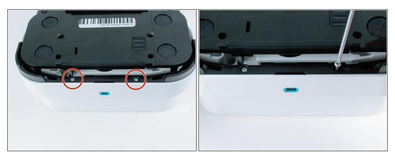
• Remove the two 22.0 mm screws on the bottom-front of the robot using a Phillips #1 screwdriver.
