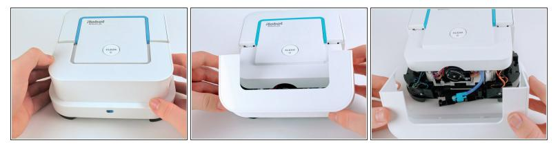
• Carefully pull back on the front shell to remove it from the robot.
