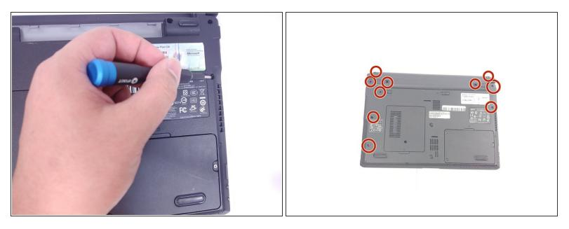
● Using the Phillips #1 screwdriver, unscrew the ten screws securing the back panel.
