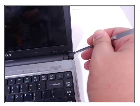
• Remove the two black connectors at the base of the screen.
