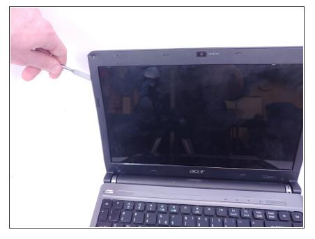
Remove the plastic siding from the screen.
