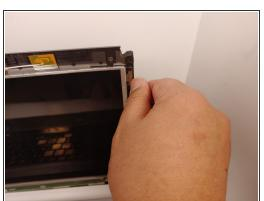
Remove the four metal bars in each corner of the screen.
