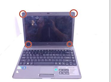
Using the Phillips #1 screwdriver, remove the four screws holding the plastic siding to the screen.
