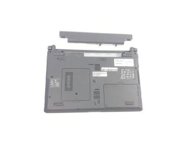
Slide the release button and remove the battery.
