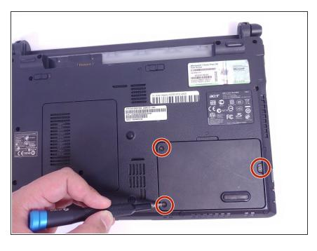
Using the Phillips #1 screwdriver, remove the three Phillips screws on the hard drive cover so the cover may be removed.
