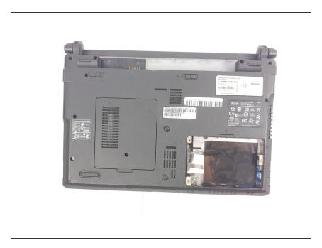
After the cover is removed, remove the hard drive from the device.
