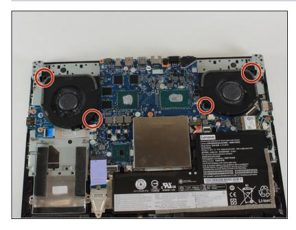
Use a JIS #1 screwdriver to remove four 4mm screws securing the fans to the device.
