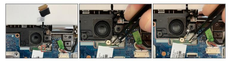
• Use the Blunt <u>Tweezers</u> to disconnect the Wireless Card Antenna Cables. Start with the cable labeled M2, which is connected to Port #2. To disconnect he cable, grab it on both sides with the tweezers and pull up.
