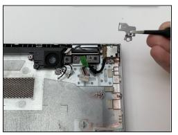
• Using the Blunt <u>Tweezers</u>, gently lift the metal piece that covers the DC Power Jack unit and the metal piece will pop out.
