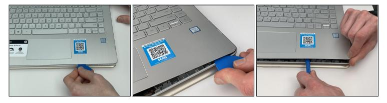
• Using the iFixit Plastic Opening Tool and the iFixit Opening Picks, work your way around the rest of the keyboard and pry it out of the base.
