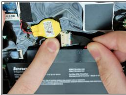
Carefully unplug the battery cable from the connector on the motherboard, using your fingers to pull the cable straight out of the port.
