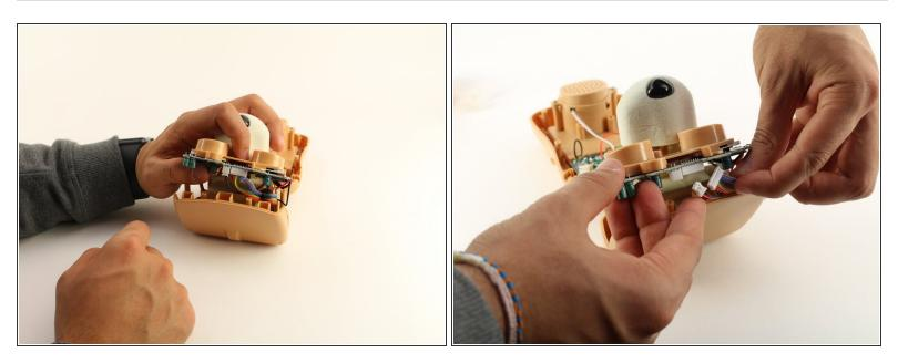
• Unplug the two sets of wires connected to the back of the eyes by using moderate to high force.
