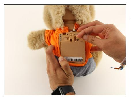
• Pull the tab outward to remove the protective plate for the batteries.
