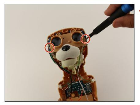
Using a Phillips #1 screwdriver, remove the two 12.5mm screws connecting the eyes to the rest of the mechanism.
