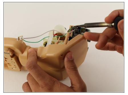
Once those wires are disconnected, desolder the wires connected from the eye motherboard.
