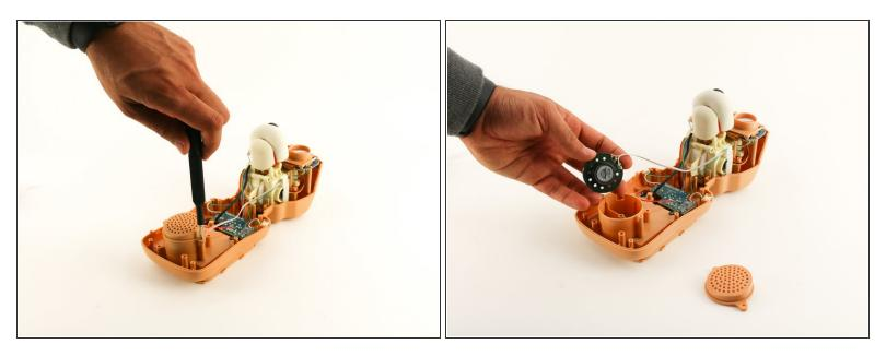
Unscrew the two 12.5mm Phillips #1 screws holding the speaker cap on and remove the speaker cap.
