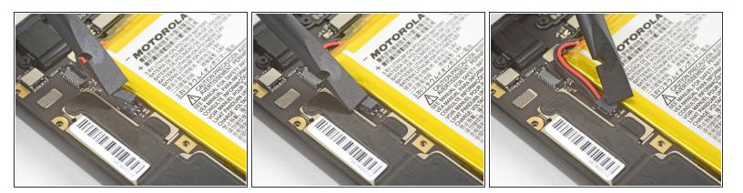
To re-connect the battery, align the connector on top of the socket, and press it down with your finger or a spudger.
