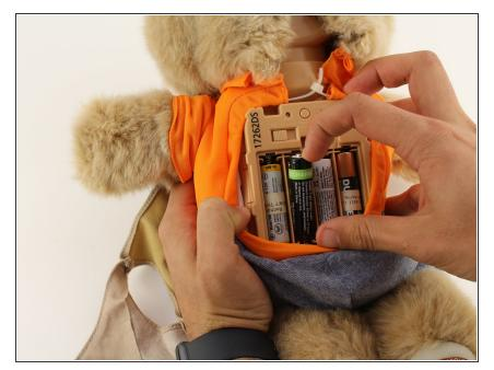
Remove all four AA batteries by pushing the positive end down and pulling the battery out toward yourself.
