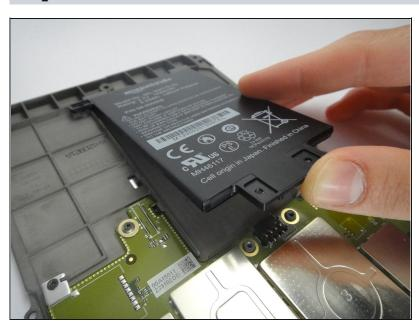
Gently lift the battery from the bottom, and slide it out of the midframe.
