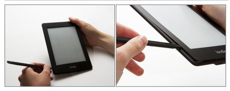
Using a spudger or plastic opening tool, gently pry the bezel from the screen. It is easier to start in the corners and work your way around the bezel.
