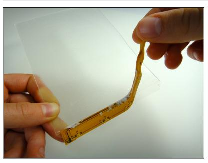
Once the outer screen is removed from the Kindle, gently use your fingers to pull off the LED lights.
