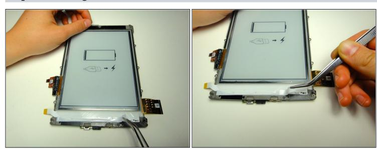
• Use a pair of <u>tweezers</u> to remove the white strip of tape that covers the LED lights.
