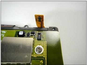
• Remove the white flex cable by gently lifting the yellow plastic connector.
