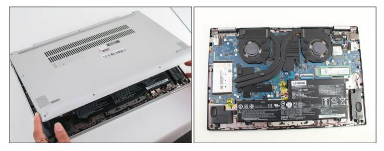
• Pry around the edges from one side to another with a plastic opening tool.
