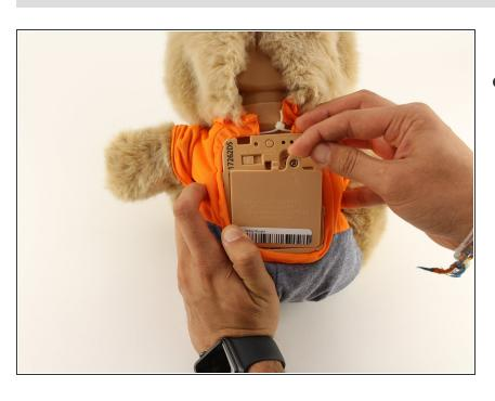
Pull the tab outward to remove the protective plate for the batteries.
