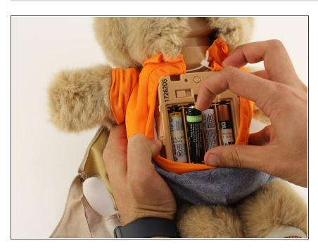
Remove all four AA batteries by pushing the positive end down and pulling the battery out toward yourself.
