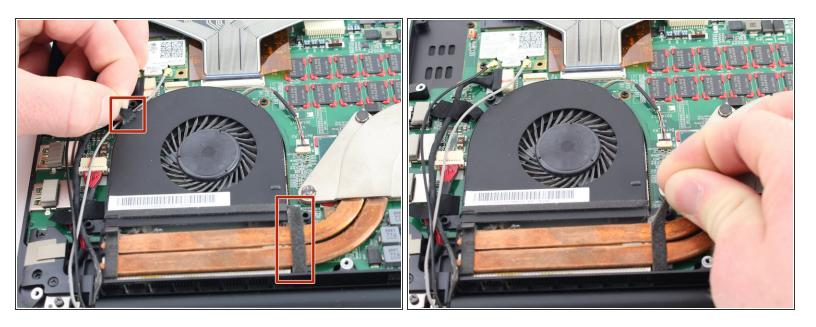
Peel back the two adhesive strips from the fan until they are removed.
