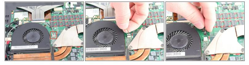
• Remove the connector by pulling it away from the motherboard with your fingers.
