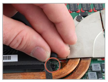
Remove the three 3mm Phillips #0 screws.
