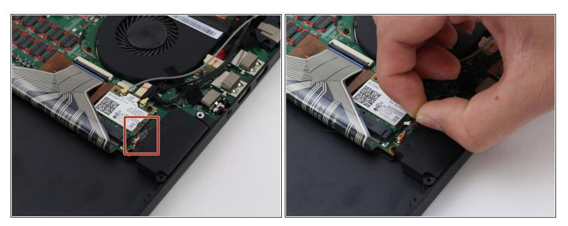
Using your fingers, gently pull on the wire connecting the speaker to the motherboard until it disconnects.
