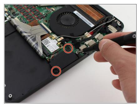
Using the Phillips #0 screwdriver, remove the two 3mm screws from the right speaker.
