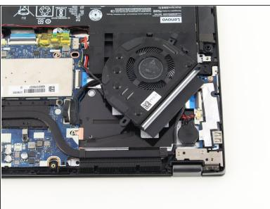
Remove the two 3.6 mm fan screws located in the top left corner of the device.
