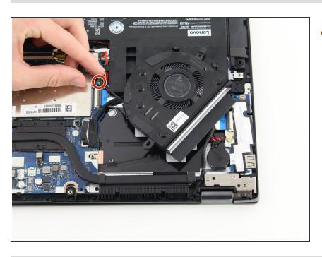
Find the black cable connecting the fan to the motherboard and gently unplug the cable to fully remove the fan.
