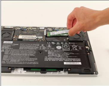
• Pull up lightly on the drive and gently pull it out of the connector.
