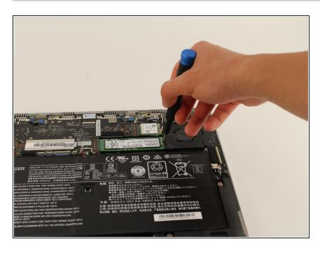
Remove the 3mm JIS #00 screw holding the storage in place.
