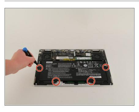
Remove the four 3 mm Phillips #0 screws holding the battery in place.
