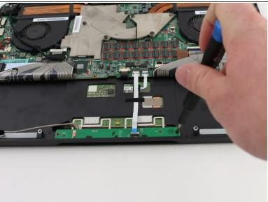
Use a Phillips #1 screwdriver to remove the two 3 mm screws holding the trackpad's circuit board to the chassis.
