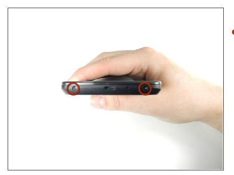
Remove the two screws from the bottom of the phone with a <u>T5 Torx</u> <u>Screwdriver</u>.
