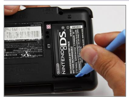
Use a plastic opening tool or spudger to pry out the battery from the bottom. If a plastic opening tool or spudger isn't available, your fingernails may work.
