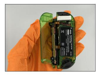
• Flip open the back shell to expose the battery.
