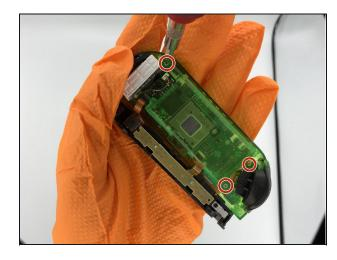
• Remove the 3 screws holding the battery casing in the shell.
