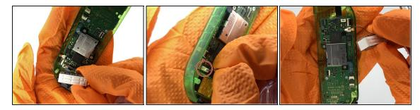
• Remove the rumble motor by disconnecting the white 2-pin connector.
