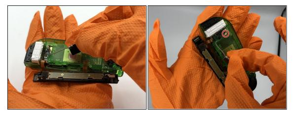
Before performing the next step, take note of how the antenna cable is seated for proper reassembly.
