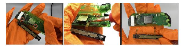
• Remove the ribbon cables connecting the rail and battery casing to the motherboard. Unlock the cables by flipping the connector upwards with a spudger, then pull the cable out of the connector.
