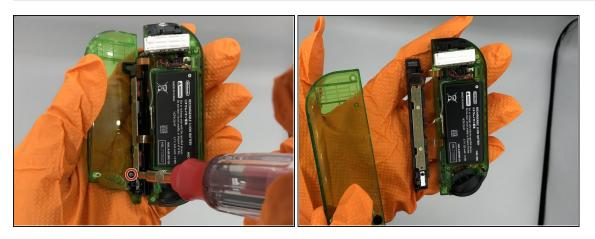
• Remove the screw connecting the rail to the back shell.
