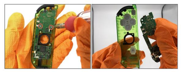
• Remove the two screws anchoring the motherboard to the shell.
