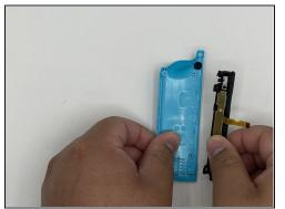
• Remove the screw holding the rail in place. Remove the rail from the back frame and set it off to the side.
