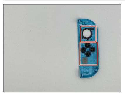
• Remove the remaining five buttons from the shell.
