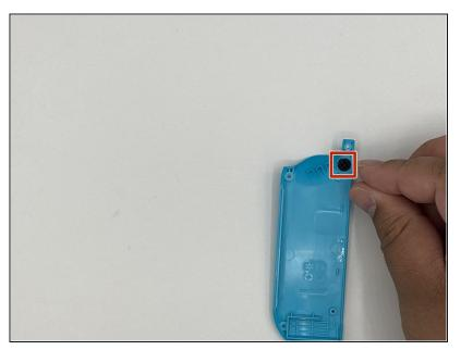
• Remove the latch button and set it off to the side.
