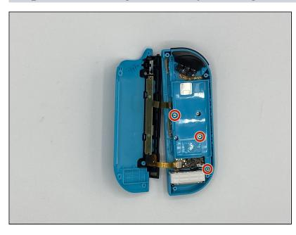
• Remove the three (3) 3½mm golden Phillips #00 screws from the midframe.
