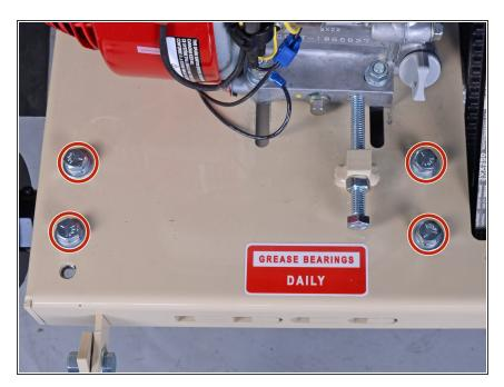
Use a 9/16-inch wrench to remove the four bolts securing the arbor assembly to the concrete saw.
