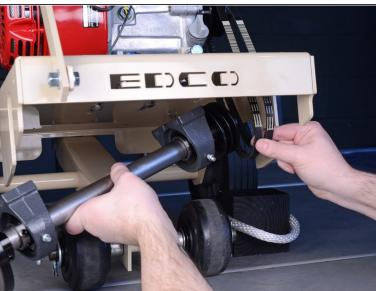
Support the arbor assembly from the bottom and tilt the left side down to remove it from the belts.
