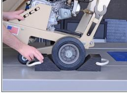
To prevent the concrete saw from rolling during service, place wheel chocks in front of and behind a rear wheel.
