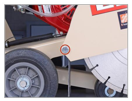
Use a 3/4-inch wrench to loosen the blade cover pivot bolt, but do not remove it.
