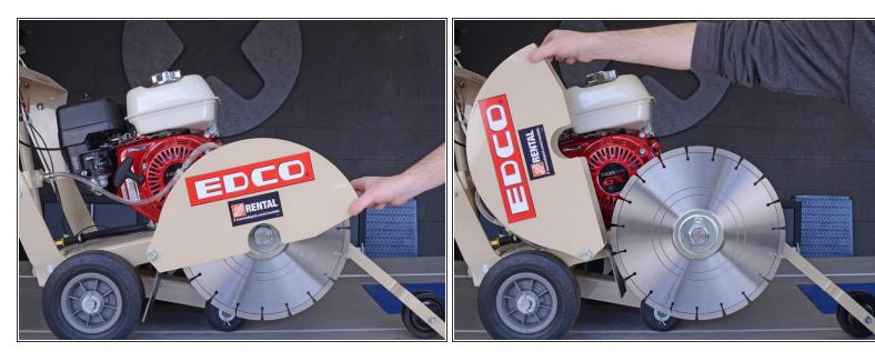
Raise the blade cover all the way up to expose the cutting blade.
