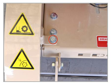
Use a 9/16-inch wrench to remove the bolt securing the blade cover.
