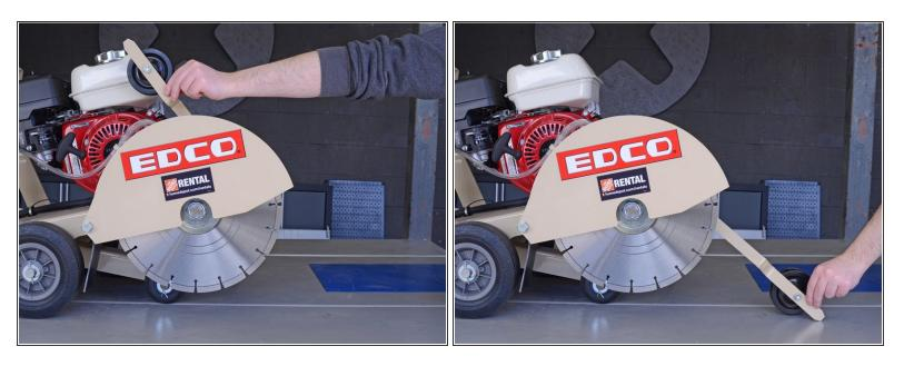
Lower the guide bar all the way down until it rests on the work surface.
