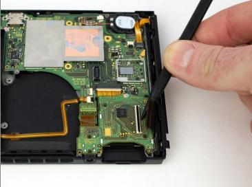
• Use the pointed end of a spudger to slide the ribbon cable out of the ZIF connector.
