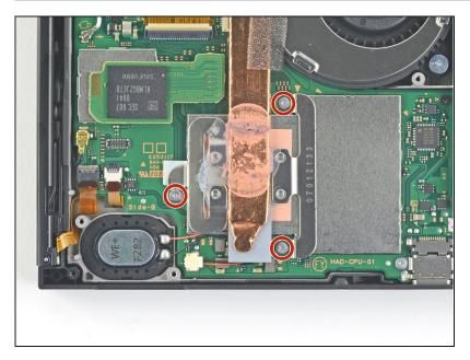
Use a JIS 000 screwdriver or an official iFixit PH 000 driver to remove the three 3 mm screws securing the heat sink to the motherboard.
