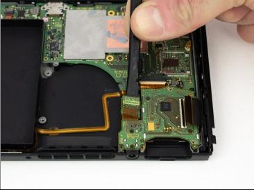
• Use the flat end of a spudger to pry the headphone jack press-fit connector straight up off the motherboard.
