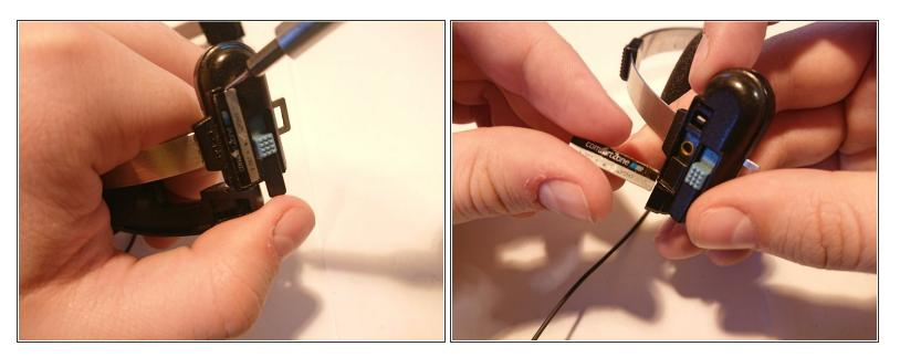
• Remove label using flat screwdriver.
