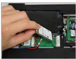
• Lift up the unattached side of the wireless card and pull out to remove.
