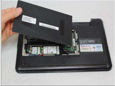
Lift the memory shield up and remove from the laptop.
