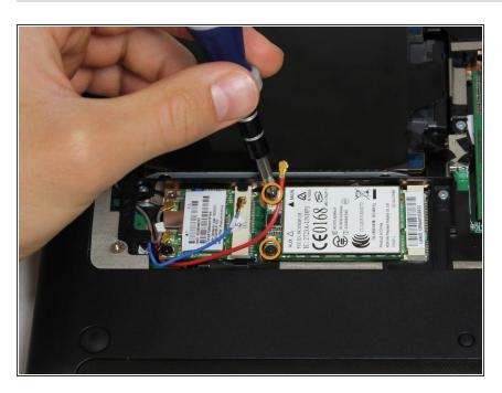
Remove the two Phillips 00 3.8mm screws attached to the wireless card.
