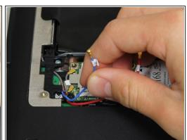
Begin by removing the red and blue wires from the wireless card.
