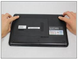
Lay the laptop on a flat surface, bottom side up and slide the two battery release latches toward the outside of the case.
