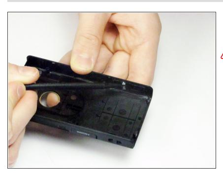
• Unclip the two plastic buttons with the spudger tool.
