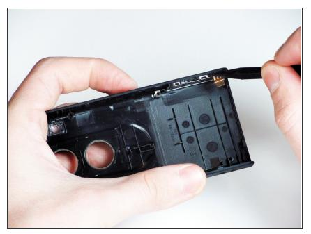
• Using a spudger, carefully remove the metal casing that is attached to the ZIF connector.
