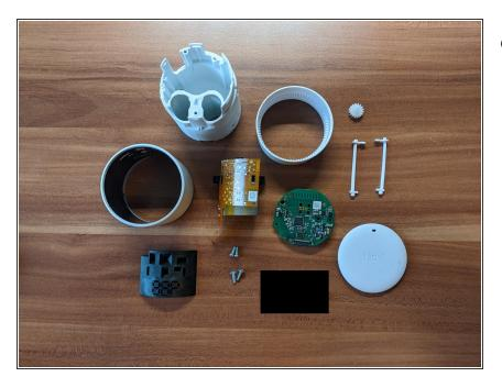
And that is it, the completly disassembled tado Smart Radiator Thermostat v3+.
