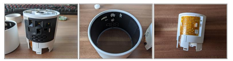
• Here you can see how the managed to implement a bent "display". The black part is made out of rubber, blocking all the light of the LEDs in the ribbon cable behind.
