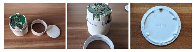
Removing the cover which has the "tado" logo embossed is the first step to getting into the thermostat.
