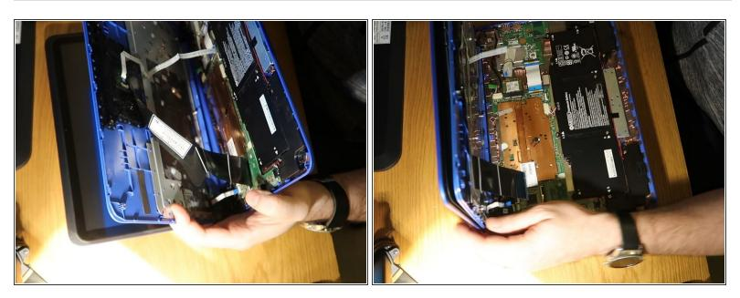
Slowley lift the top case/keyboard upwards and disconnect the three ribon cables.
