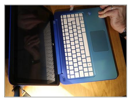
Carefully pry up around the edges of the laptop. Take your time around the ports as they can easily get damaged.
