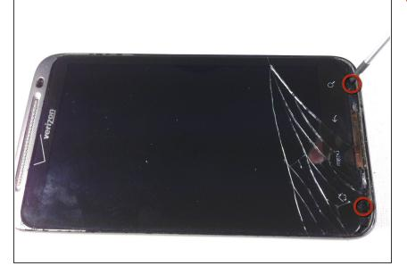
• Remove the two Phillips screws where the plastic cover was.
