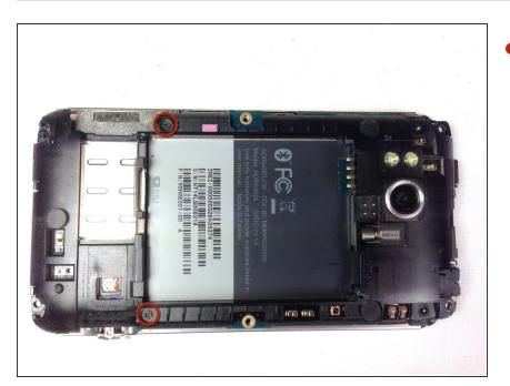
Remove the two Phillips screws securing rear inner frame to device.
