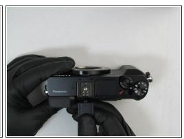
Remove the plastic hot shoe cover by sliding it towards the rear of the camera.
