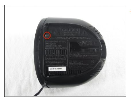
On the bottom of the clock locate and unscrew the single 2mm Phillips screw from bottom of the clock.
