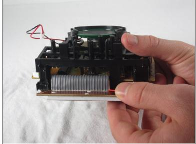
Applying a bit of pressure at each of the contact points (illustrated by red circles), disconnect the display from the plastic housing.
