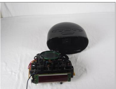
Get a firm grip on the outside of the clock and a firm grip on the hardware on the inside of the the clock like so and pull the hardware out from the outside of the clock.
