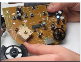
• Gently, pull the tuner wheel up and away from the motherboard.
