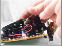
Using your fingers, pull the power cord connector, outlined in the picture with a red rectangle straight up to disconnect from the alarm clock.
