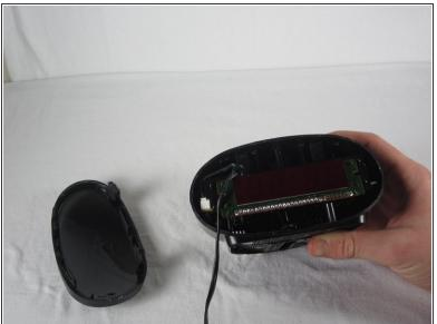
Using a moderate amount of force, position the screwdriver in the crack between the front screen and the main body of the clock (as shown) and push the screen away from the main body of the clock.
