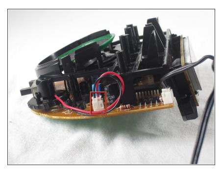
Just as before, pull the speaker plug directly up to remove the plug from the motherboard.
