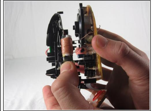
**⚠ Do not pull the plastic frame and motherboard apart too hard or the motherboard and plastic frame will not go back together.**
