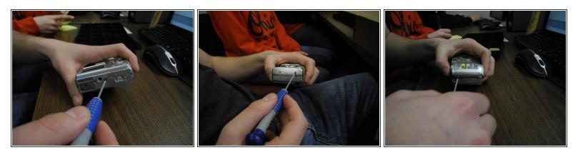
• Remove the screws from the bottom, right, and left side of camera.
