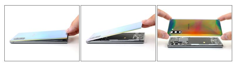
Lift up and remove the back panel.
