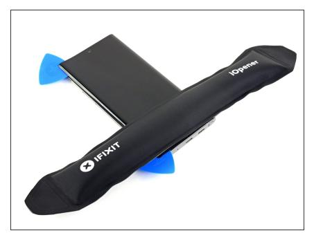
Prepare an iOpener and apply it to the bottom edge of the phone for one minute.
