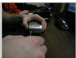
Remove the screws from the bottom, right, and left side of camera.
